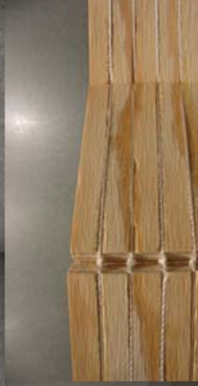
How can pieces of wood become hinged? This was the focus of this piece, where slices were cut out of the surface of the plywood pieces and string was used to hinge them together.
